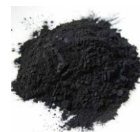
Fig. 2. Photograph of activated carbon derived from the bark of Anacardium Occidentale Tree .
