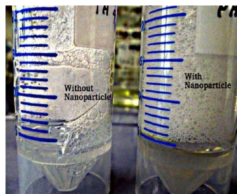
Fig. 6. Samples of 0.03 wt % alpha olefin sulfonate foam with (right) and without (left) nano ash (<0.05 wt %) after addition of 1 mL of Shell Ondina 919 to the generated foam (Reproduced from Eftekhari et al., 2015).
