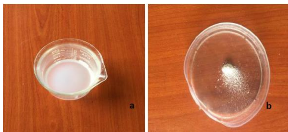
Fig. 1. (a) Sol-gel Formation in \text{SiO}_2 and (b) \text{SiO}_2 Nps synthesized
