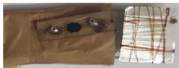
Fig. 5. Gas Sensor fabricated for sensing of NH 3 gas
